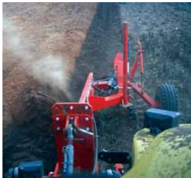
Light subsoil (left) buries the dark topsoil (right).
