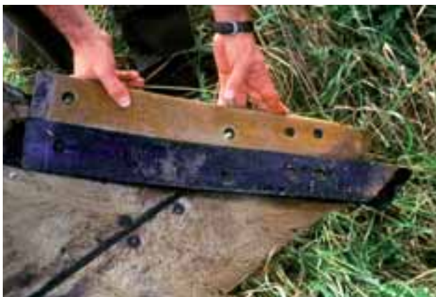
Wear on the points is greater on sandy subsoils.
